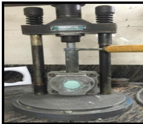
Figure 6: Special Flask under Hydraulic Pressure during Injection Molding
