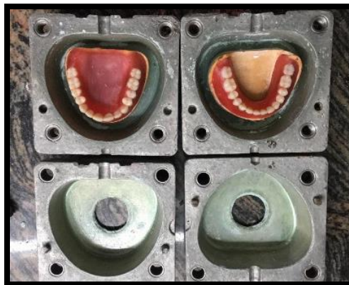
Figure 5: CD Samples Ready to be Flaked in Special Flask Designed for Injection Molding
