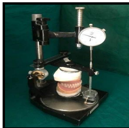
Figure 9: Articulator on Measuring device with One of the Injection Molded Denture Showing No Deflection on Micrometer
