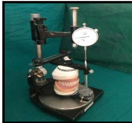
Figure 8: Articulator on measuring device with One of the Compression Molded Denture Showing Deflection on Micrometer
